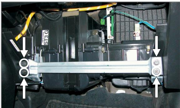
**EN** Remove the protecting device
