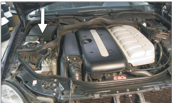
**EN** Open the front bonnet. Pollen filter is located behind the engine chamber
