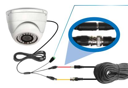
Connect the camera's DC and BNC socket cable to the extension cable's DC and BNC plugs
