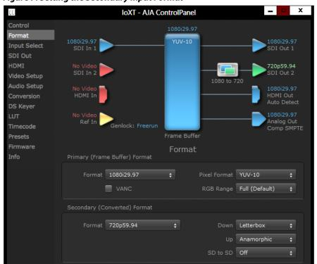
Figure 7. Setting the Secondary Input Format
