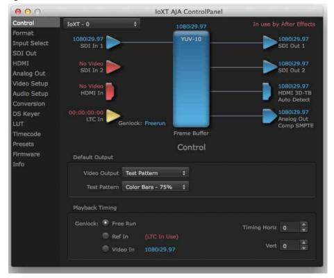
Figure 10. AJA Control Panel, Control Screen
