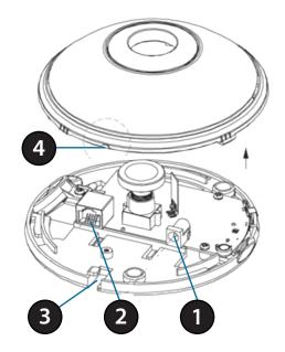
You can access the inside of the DCS-6010L by rotating the camera cover counter-clockwise, then lifting it off of the camera.
