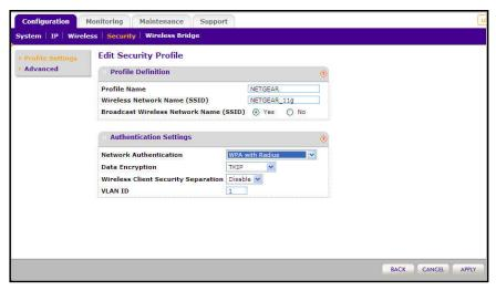
Figure 20. Configure WPA with RADIUS
