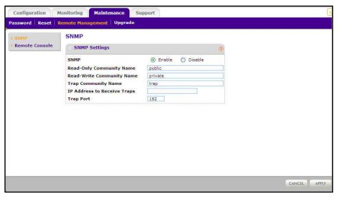
Figure 27. Configure SNMP settings
