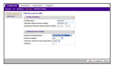
Figure 21. Configure WPA2 with RADIUS
