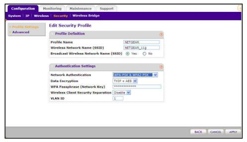
Figure 25. Configure WPA-PSK and WPA2-PSK
