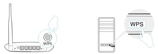
2. Within 2 minutes, press and hold the WPS button on the adapter until WPS Tool opens in the lower right corner of your computer.
