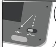
On the back of the Star 05, you'll find a small pinhole to the left of the Off/On switch.
