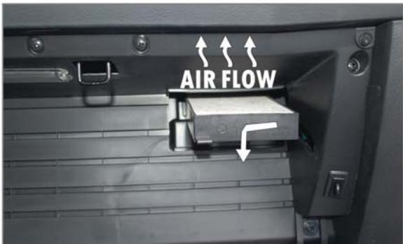
Carefully remove the second filter, install the new one and perform the previous actions in the opposite order
