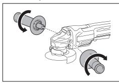
Installing or removing wheel guard (For depressed center wheel, flap disc, flex wheel, wire wheel brush / abrasive cut-off wheel, diamond wheel)
