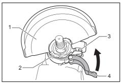
▶ 1. Wheel guard 2. Bearing box 3. Screw 4. Lever
