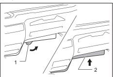
1. Lock-off lever 2. Switch lever
