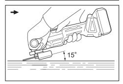
Turn the tool on and then apply the wheel or disc to the workpiece.
