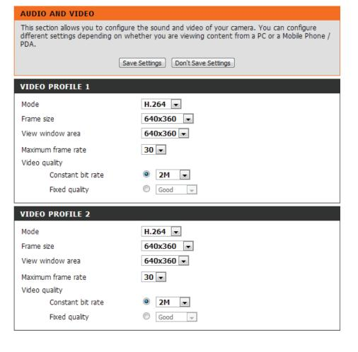
Video Quality: This limits the maximum frame rate, which can be combined with the "Fixed quality" option to optimize the bandwidth utilization and video quality. If fixed bandwidth utilization is desired regardless of the video quality, choose "Constant bit rate" and select the desired bandwidth.
