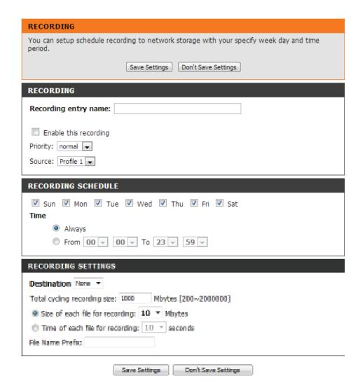
Total cycling Please input a HDD volume between 1MB and 2TB recording size: for recording space. The recording data will replace the oldest record when the total recording size exceeds this value. For example, if each recording file is 6MB, and the total cyclical recording size is 600MB, then the camera will record 100 files in the specified location (folder) and will then delete the oldest file and create new file for cyclical recording.
