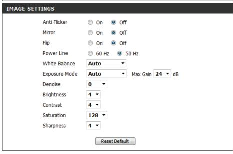
**Exposure Mode:** Changes the exposure mode. Use the drop-down box to set the camera for Auto, Indoor, Outdoor, Night Environments, or to Moving to capture moving objects. The Low Noise option will focus on creating a high-quality picture without noise. You can also create 3 different custom exposure modes. The Max Gain setting will allow you to control the maximum amount of gain to apply to brighten the picture.
