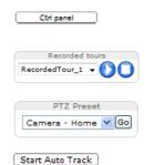
Click the **Ctrl panel** button to open the PTZ control panel which provides additional PTZ controls. User-defined buttons can also appear in the Control panel. See *Controls on page 28*.
