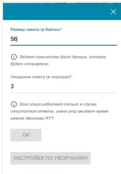
The screenshot shows a settings window titled 'Система / Пинг' (System / Ping). It contains two input fields: 'Размер пакета (в байтах)\*' (Packet size in bytes) with the value '56' and 'Ожидание ответа (в секундах)\*' (Response time in seconds) with the value '3'. Below each field is an information icon and a descriptive note. At the bottom, there are two buttons: 'ОК' (OK) and 'НАСТРОЙКИ ПО УМОЛЧАНИЮ' (Default Settings).
