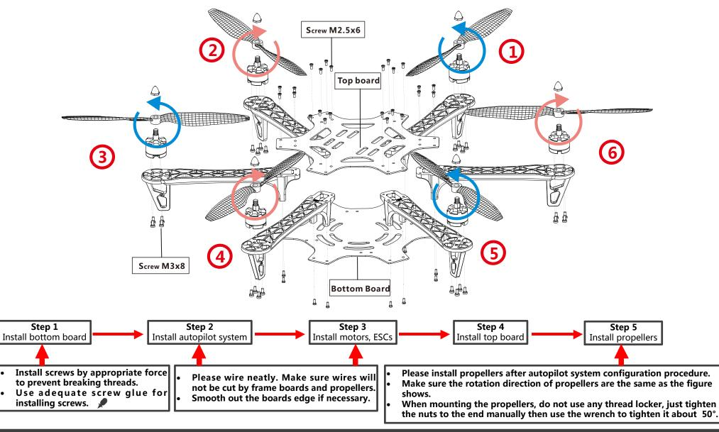
In up figure, arms (0) front of craft, arms (0) are back of craft. See from top, motors on arms (0) rotate counter-clock wise, use propellers 1038; motors on arms (0) rotate clock wise, use propellers 1038R.
