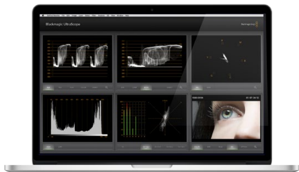
Blackmagic UltraScope的“Full Screen” (全屏)视图 Blackmagic UltraScope让您在Blackmagic Cinema Camera或 Production Camera 4K上精确监看视频和音频电平。
