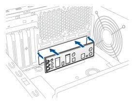
Place the motherboard into the chassis, ensuring that its rear I/O ports are aligned to the chassis' rear I/O panel.
