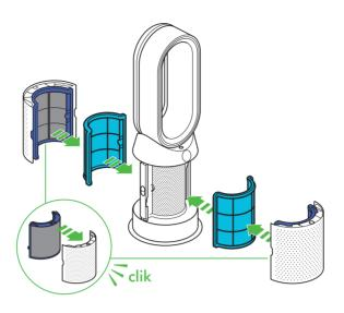
Your machine comes with a permanent Dyson Cryptomic™ filter and a Combination filter.
