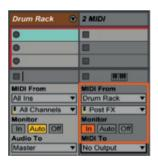
Finally, in the 'MIDI To' choosers select Launchpad Pro Output in the top, and Ch. 6 (User Mode's default channel) on the bottom.
