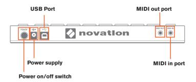
Troubleshooting: If your Launchpad Pro is not working properly, it could be an issue with your USB Hub, computer's USB port, or even the USB cable you are using. Please use the USB cable included in the box. If this still does not fix your issue, connect the included 12V DC power supply.
