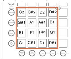
E2 to G3 are then playable in the 4x4 area directly above C1 to D#2. Meanwhile, G#3 to B4 continues in the lower-right 4x4 area, and C5 to D#6 are playable in the upper-right 4x4 area of the pad grid. The following diagram illustrates this:
