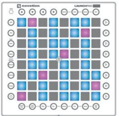
By default, the pad in the lower-left corner of the 8x8 note grid plays the note C1-the blue and pink pads therefore outline a C major scale. You can transpose this layout up or down in semitones by
