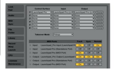
Track On sets the Launchpad Pro as an Input device to play MIDI tracks (instruments and drums) in Live, and as and Output device to see played and recorded notes fed-back to the pad LEDs.
