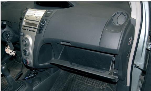
EN Open the glove locker, Filter is located behind the glove compartment
