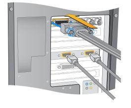
Attach the supplied DeckLink breakout cable to the DeckLink card. The DeckLink HD Extreme 2 card also includes a HDMI bracket as pictured above.
