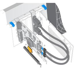
Install a DeckLink PCIe x1 or x4 lane card in a compatible PCI Express slot as shown in the above picture. The DeckLink HD Extreme 2 also has an HDMI bracket, which installs in any spare port, and connects to the rear of the card with the supplied HDMI cables.
