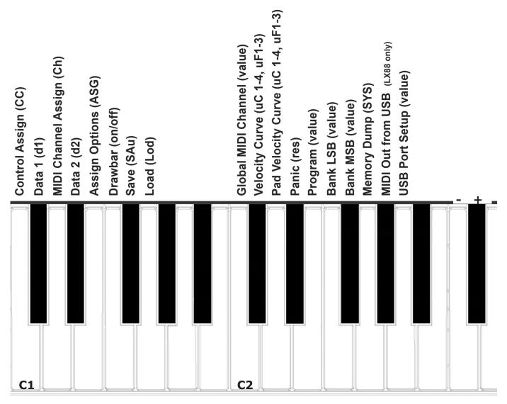
Menu keys are the same for both Impact LX49, LX61 and LX88 but value entry using the keyboard is one octave higher on LX61 and LX88. Refer to the screen printing on the unit to see which keys to press to enter values.
