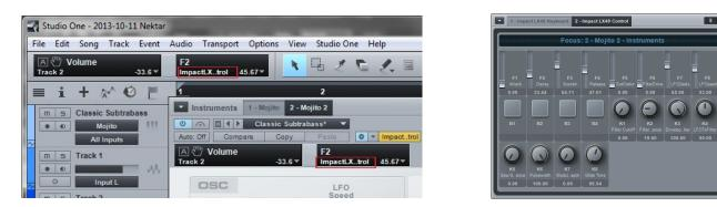
The Focus window will show you the name of each parameter assigned to Impact LX's Instrument preset controls at any one time and their current value.
