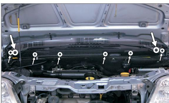
**EN** Dismount the wiper and loosen the screws of the screen under the windshield
