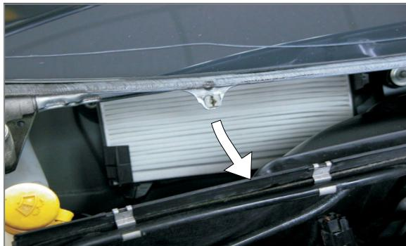
**(EN)** Open the locks of the pollen filter. Remove the filter from the frame, put in the new one and perform the previous actions in the opposite order
