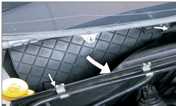
**(EN)** Open the locks which hold the filter housing. Remove the housing
