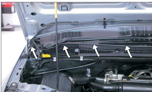
**EN** Remove the rubber seal
