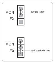
Fig. 5.1: Modification MON/FX "pre fader" > "post fader"0
