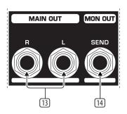
Fig. 2.4: MAIN OUT and MON OUT SEND connectors
