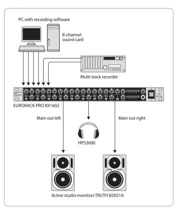
Fig. 3.3: Monitoring multi-track recorders or multi-channel sound cards
