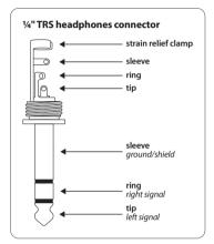
Fig. 4.3: 1/4" TRS connector for headphones operation
