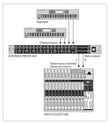
Fig. 3.1: Keyboard sub-mix using the RX1602
